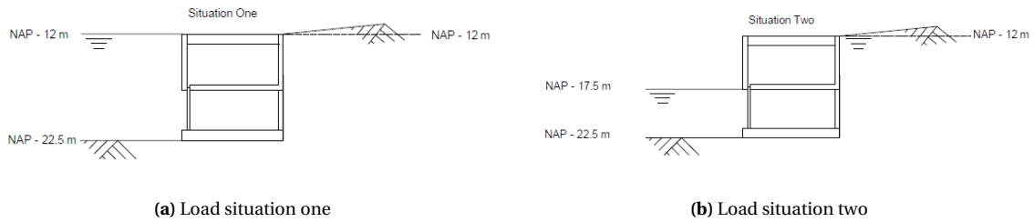
Figure 6.7: The load situation for the concept Siphon
