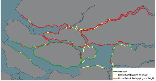
(b) Delta21, failure probability of Europoort barrier of 1/1000 per closure and 1 meter sea level rise.
