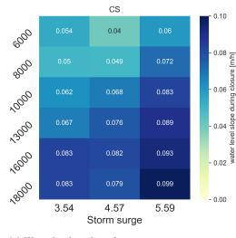
(a) Water level gradient for current system.
