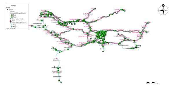
Figure 3.5: The RMM-model in SOBEK3. The arrows and green dots represent the branches and nodes respectively. Moreover, all structures are included. The boundaries on the east side of the domain are governed by the discharge of the rivers Lek, Waal and Maas. The boundary nodes on the west side are governed by the water level at the North Sea.
