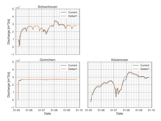
Figure 4.13: Discharges for both configurations during a storm with a Rhine discharge  $(Q_{Lobith})$  of 10 000 m<sup>3</sup>/s and storm surge (L) of 3.54 m. Locations are in the discharge dominant area.
