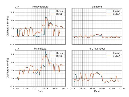
Figure 4.9: Discharges for both configurations during a storm with a Rhine discharge ( $Q_{Lobith}$ ) of 10 000 m<sup>3</sup>/s and storm surge (L) of 3.54 m. Locations are in the flood storage dominant area.
