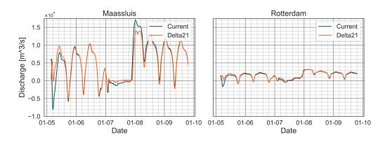
Figure 4.5: Discharges for both configurations during a storm with a Rhine discharge  $(Q_{Lobith})$  of 10 000 m<sup>3</sup>/s and storm surge (L) of 3.54 m. Locations are in the storm surge dominant area.
