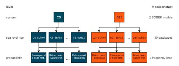
Figure 3.7: Graphical representation of the simulation approach. The blue boxes indicate simulations in which the current system is used. The orange boxes represent simulations with the properties of Delta21. For each step of sea level rise 0f 0.5 meters, 164 simulations are made corresponding to 9 discharges, 6 storm surges and three operation states of the Europoort barrier.
