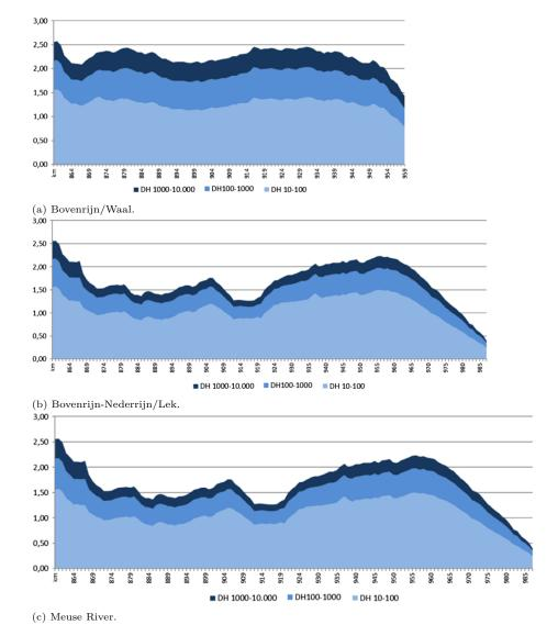
Figure 2.3: Cumulative decimation heights for the Bovenrijn-Nederrijn/Lek, Bovenrijn-Waal and Meuse River. The figure depics the differences in flood water levels with probabilities of occurrence ranging between 1:10 to 1:10,000 per year. On the x-axis, the chainage of the corresponding branch is denoted (Hegnauer et al., 2014; Klijn et al., 2018).
