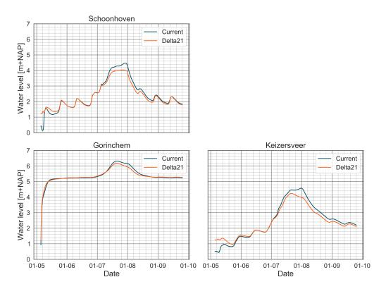
Figure 4.12: Water levels for both configurations during a storm with a Rhine discharge  $(Q_{Lobith})$  of 10 000 m<sup>3</sup>/s and storm surge (L) of 3.54 m. Locations are in the discharge dominant area.
