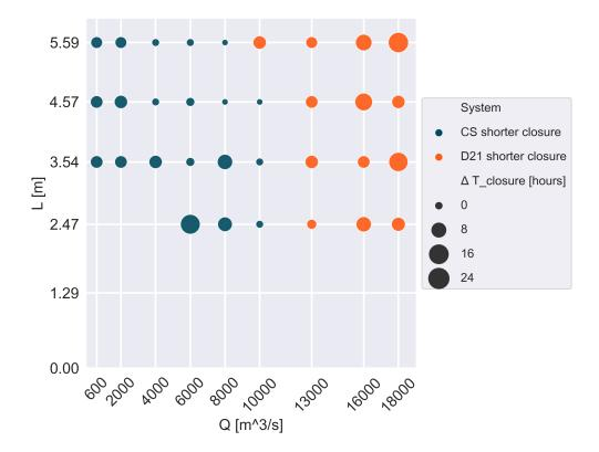
Figure 4.22: Difference in closure duration of the current configuration and a configuration with Delta21. The size of the circles indicates difference in number of hours. An blue circle corresponds to a shorter closure of the current configuration, an orange circle represents an shorter closure for Delta21.
