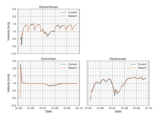
Figure 4.14: Velocities for both configurations during a storm with a Rhine discharge  $(Q_{Lobith})$  of 10 000 m<sup>3</sup>/s and storm surge (L) of 3.54 m. Locations are in the discharge dominant area.
