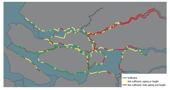
(a) Current system, failure probability of Europoort barrier of 1/100 per closure and 0 meter sea level rise.
