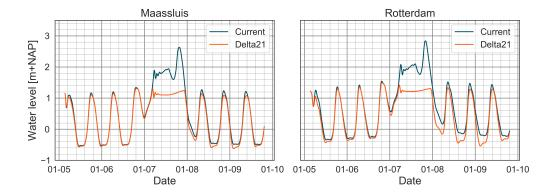
Figure 4.4: Water levels for both configurations during a storm with a Rhine discharge  $(Q_{Lobith})$  of 10 000 m3)/s and storm surge (L) of 3.54 m. Locations are in the storm surge dominant area.
