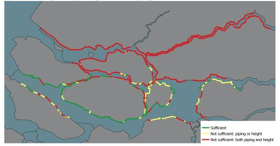
(c) Delta21, failure probability of Europoort barrier of 1/100 per closure and 2 meter sea level rise.
