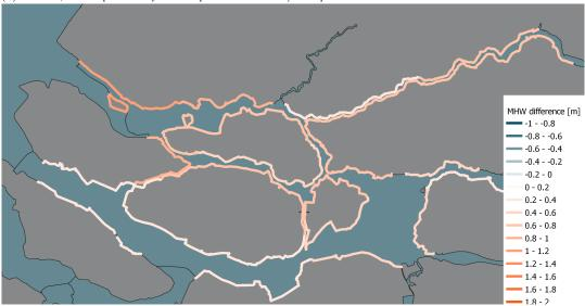
(b) Delta21, failure probability of Europoort barrier of 1/1000 per closure and 1 m sea level rise.
