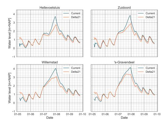
Figure 4.8: Water levels for both configurations during a storm with a Rhine discharge  $(Q_{Lobith})$  of 10 000 m<sup>3</sup>/s and storm surge (L) of 3.54 m. Locations are in the flood storage dominant area.
