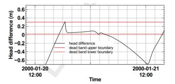
Figure B.2: Illustration of dead-band control of the Haringvliet sluices triggered by the head difference (Deltares, 2019).
