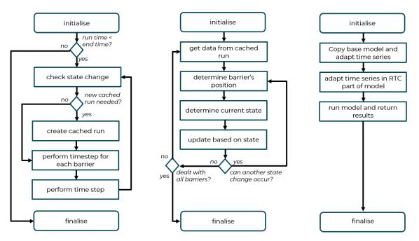
Figure B.3: Various loops of Singlerunner. The left loop investigates whether a new cached run is needs, the loop in the middle updates the state and corresponding position of the barrier and the right loop writes the results of the RTC to SOBEK (Adjusted from Deltares (2018)).
