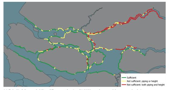
(a) Delta21, failure probability of Europoort barrier of 1/1000 per closure and 0 meter sea level rise.
