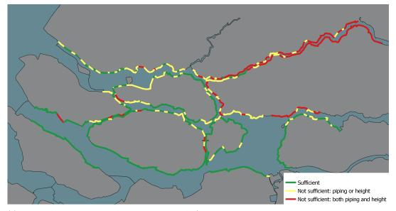
(a) Delta21, failure probability of Europoort barrier of  $1/100~{\rm per}$  closure and 0 meter sea level rise.
