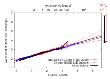
(a) Gumbel plot for water levels at Hoek van Holland. Observations of water levels and the corresponding generalised extreme value fit are shown in black. The blue and red dots indicate data from different WAQUA computations (Sterl et al., 2009).
