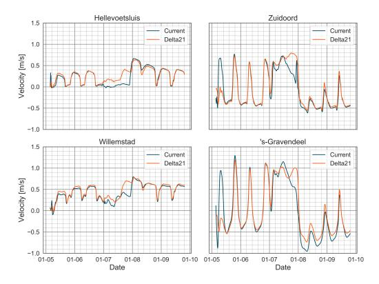
Figure 4.10: Velocities for both configurations during a storm with a Rhine discharge ( $Q_{Lobith}$ ) of 10 000 m<sup>3</sup>/s and storm surge (L) of 3.54 m. Locations are in the flood storage dominant area.
