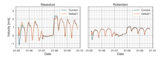
Figure 4.6: Velocities for both configurations during a storm with a Rhine discharge  $(Q_{Lobith})$  of 10 000 m<sup>3</sup>/s and storm surge (L) of 3.54 m. Locations are in the storm surge dominant area.
