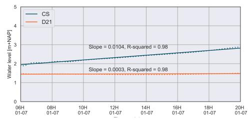
(b) Water level at Rotterdam during the closure of the Europoort barrier. The red square of the upper plot corresponds with the boundaries of this plot. A linear regression line is fitted through the observation points of the simulation, including the slope [m/h] and R-squared.
