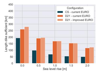
Figure 6.11: Kilometers dike that meet the norm for three different configurations. For different steps of sea level rise, the length of dikes that meet the norms for piping or height are depicted. The current system is depicted in blue and Delta21 is rendered in orange. For Delta21, a distinction is made between the current failure probability (1/100 per closure) and an improved failure probability (1/100 per closure) of the Europoort barrier. The total length of dikes in the domain is 484 km.
