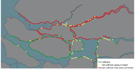
(b) Delta21, failure probability of Europoort barrier of 1/100 per closure and 1 meter sea level rise.
