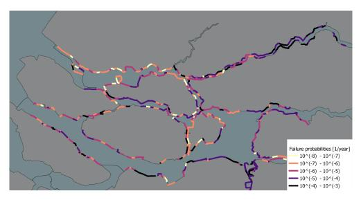
Figure 6.2: Failure probabilities for dike sections in the Rhine-Meuse estuary. Light coloured lines indicate a low failure probability, dark lines correspond to a higher failure probability. This map only provides information about the failure probability, not whether this probability meets the norm. Note that the interval of the classes is logarithmic (Based on data of Vergouwe (2015)).
