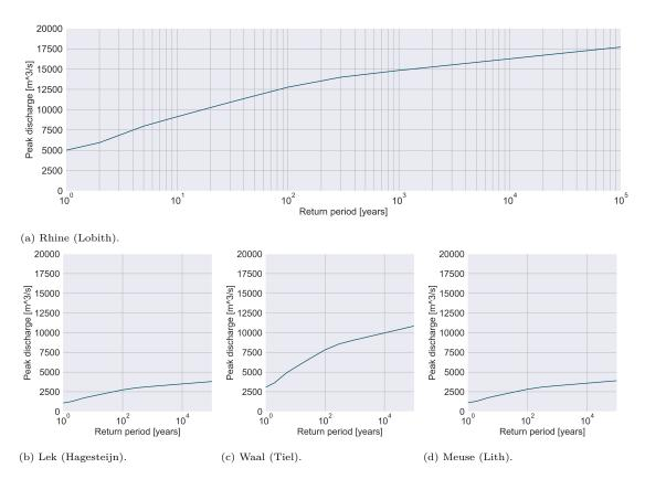
Figure 3.2: Frequency discharge curves for the Rhine branches and the Meuse. In the top graph the frequency discharge curve of the Rhine at Lobith is presented. In this research, the discharge at the Lek, Waal en Meuse river were coupled directly and is confirm WBI-2017 (Hegnauer et al., 2015; Agtersloot and Paarlberg, 2016).
