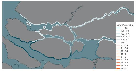
(a) Delta21, failure probability of Europoort barrier of 1/100 per closure and 0 m sea level rise.
