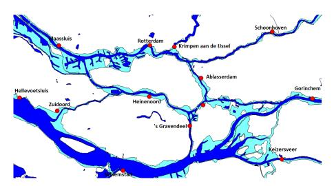
Figure 4.2: Selected locations in the domain. The locations correspond to the location mentioned in Table 4.1. The locations belong to a particular dike section. The water level, discharge, water velocity are retrieved from the nearest sobek node.
