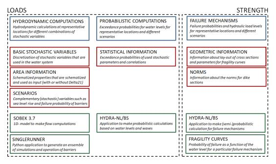
Figure 3.1: Structure of modelling approach. The blue boxes indicate the different steps undertaken in this research. The results of the hydrodynamic computations, probabilistic computations and failure mechanisms are discussed in Chapter 4, 5 and 6 respectively. The boxes with a red outline indicate which information serves as input, where the green boxes represent the used application or method.
