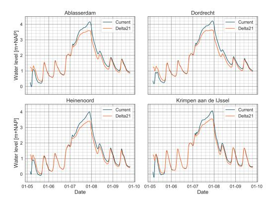
Figure 4.16: Water levels for both configurations during a storm with a Rhine discharge  $(Q_{Lobith})$  of 10 000 m<sup>3</sup>/s and storm surge (L) of 3.54 m. Locations are in the transition area.
