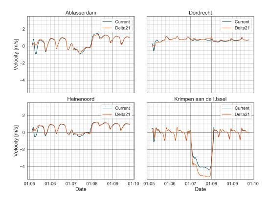
Figure 4.18: Velocities for both configurations during a storm with a Rhine discharge  $(Q_{Lobith})$  of 10 000 m<sup>3</sup>/s and storm surge (L) of 3.54 m. Locations are in the transition area.
