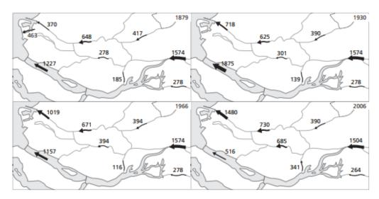
Figure 2.1: Division of mean river discharge (in  $m^3/s$ ) over channels in the RMD over the past century (Huismans and Hoitink, 2017). Major changes in discharge can be observed in the Nieuwe Waterweg and Haringvliet.
