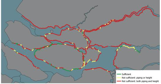
(b) Current system, failure probability of Europoort barrier of 1/100 per closure and 1 meter sea level rise.
