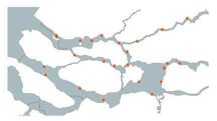
Figure 6.4: 24 locations throughout the domain for which the relative change in failure probability is computed. Each location represents a particular dike section, which in turn represents one of the segment in the Rhine-Meuse estuary (Table G.1).
