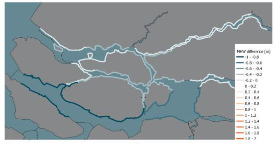
(a) Delta21, failure probability of Europoort barrier of 1/1000 per closure and 0 m sea level rise.
