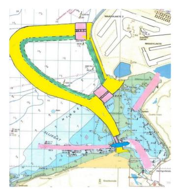
Figure 2.5: Illustration of the Delta21 plan (Delta21, 2019). The energy storage lake is constructed within the yellow dike sections. Between the Harinvlietsluices (bottom right) and the energy storage lake, a tidal lake is created. This tidal lake is connected to the North Sea with a storm surge barrier in between.
