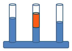
Figure 16.3: Illustration of communicating vessels.
