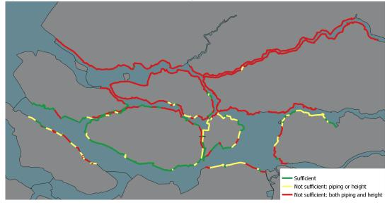
(c) Delta21, failure probability of Europoort barrier of 1/1000 per closure and 2 meter sea level rise.
