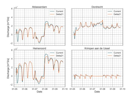
Figure 4.17: Discharges for both configurations during a storm with a Rhine discharge  $(Q_{Lobith})$  of 10 000 m<sup>3</sup>/s and storm surge (L) of 3.54 m. Locations are in the transition area.
