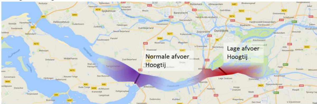
Figure 7: The line of 300 mg Cl-/l (0.54 ppt) is shown to imply to which point the brackish water will reach. At normal river discharge and high tide (“Normale afvoer, Hoogtij”) the purple line is given. At low river discharge and high tide (“Lage afvoer, Hoogtij”) the red line is given. The gradient given next to the lines shows the uncertainty in the model. Figure taken from Wijsman et al., (2018)
