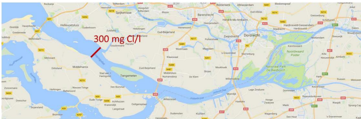
Figure 5: The line of 300 mg Cl/l (or 0.54 ppt) is shown to imply to which point the brackish water will reach. West of the line the salinity might be higher, east of the line the salinity should be lower. Figure taken from Wijsman et al., (2018)
