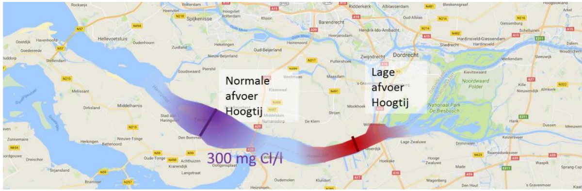
Figure 6: The line of 300 mg Cl-/l (0.54 ppt) is shown to imply to which point the brackish water will reach. At normal river discharge and high tide (“Normale afvoer, Hoogtij”) the purple line is given. At low river discharge and high tide (“Lage afvoer, Hoogtij”) the red line is given. The gradient given next to the lines shows the uncertainty in the model. Figure taken from Wijsman et al., (2018)
